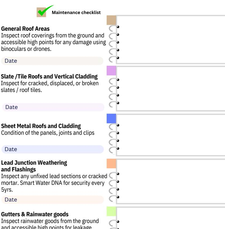
and accessible high points for leakage during wet weather. Check for blockages in gutters, hoppers and downpipes where accessible. Pay attention to heavy moss and vegetation as they can cause water ingress and dampen internal walls. Regular checks can prevent damage.
